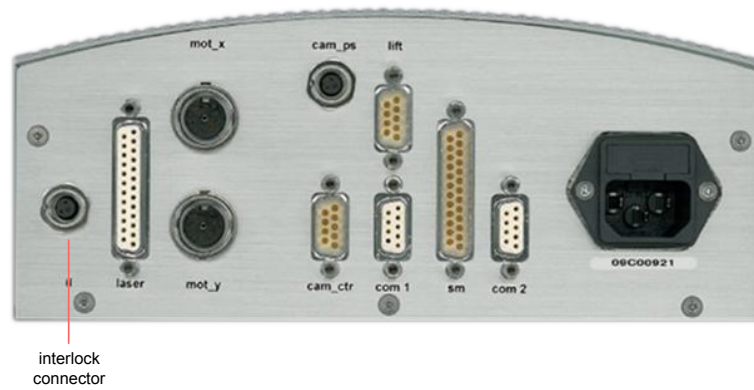
(c) Legacy controller rear side
