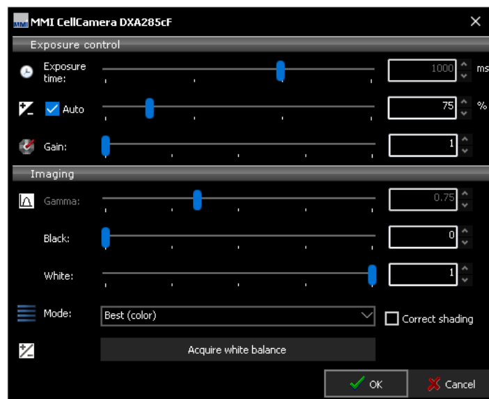
Figure 5.5: Camera settings for mmi CellCamera models
