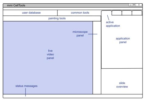
Figure 3.1: Structure of the mmi CellTools user interface
