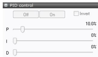
**Figure 6.30:** The PID control section appears for systems equipped with the PID optical trap controller.
