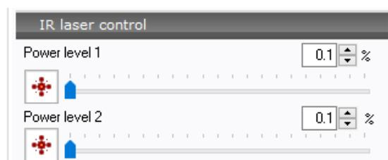
**Figure 6.2:** Power controls for the IR laser
